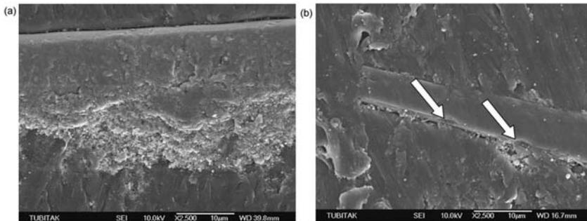
**Figure 5.** SEM micrographs of: (a) GF- and (b) CF-reinforced composite surfaces eroded at contact angle of  $30^\circ$  for 7 h.
