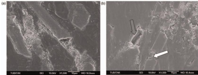
**Figure 7.** SEM micrographs of: (a) GF- and (b) CF-reinforced composite surfaces eroded at contact angle of  $60^\circ$  for 7 h.
