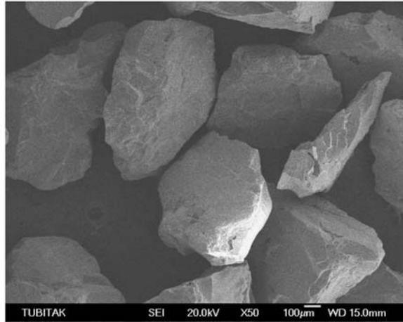
**Figure 2.** Scanning electron micrograph of aluminum oxide (500–710  $\mu\text{m}$ ).
