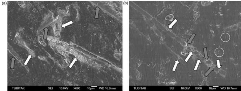
**Figure 9.** SEM micrographs of: (a) GF- and (b) CF-reinforced composite surfaces eroded at contact angle of  $45^\circ$  for 7 h.
