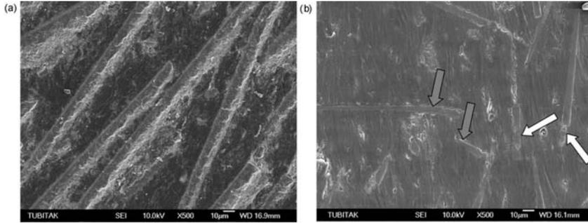
**Figure 6.** SEM micrographs of: (a) GF- and (b) CF-reinforced composite surfaces eroded at contact angle of  $15^\circ$  for 7 h.
