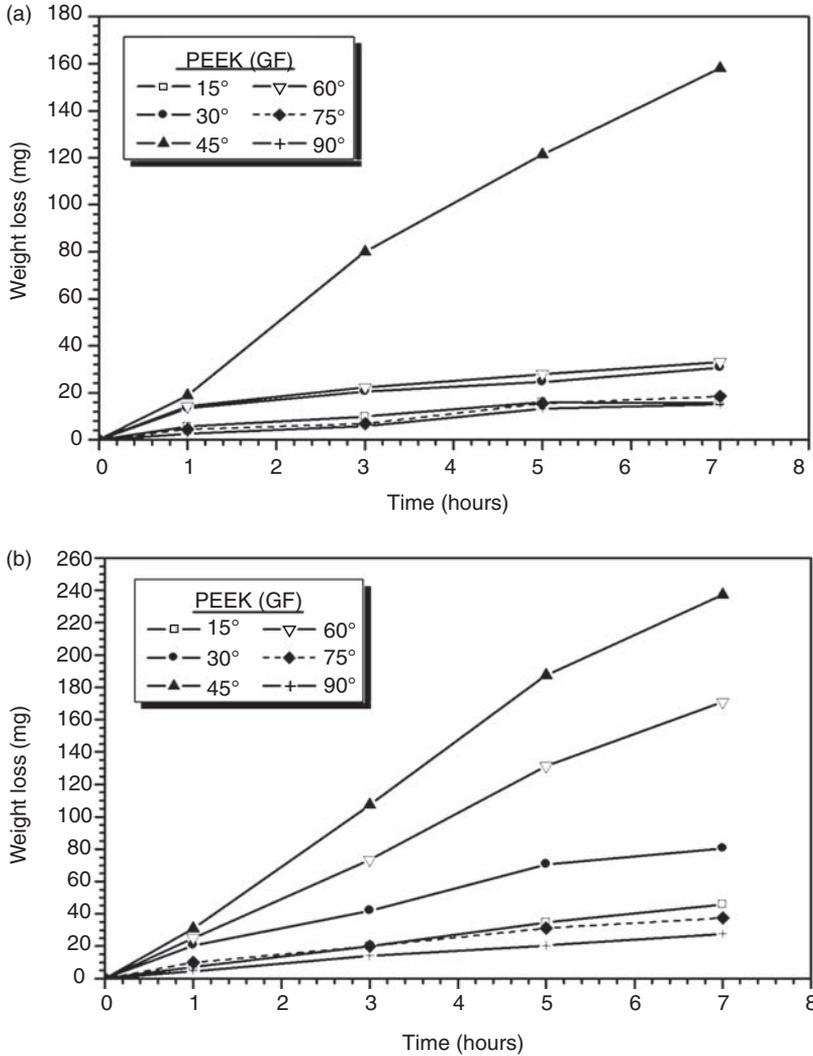
**Figure 3.** Cumulative weight loss values of samples as a function of wear time: (a) GF-reinforced PEEK and (b) CF-reinforced PEEK.
