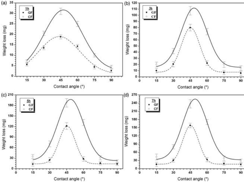
**Figure 4.** Weight loss values of the samples as a function of contact angle: (a) 1 h, (b) 3 h, (c) 5 h, and (d) 7 h erosion times.
