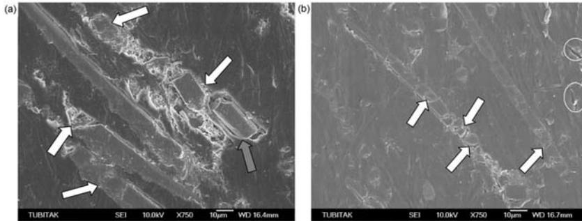
**Figure 8.** SEM micrographs of: (a) GF- and (b) CF-reinforced composite surfaces eroded at contact angle of  $45^\circ$  for 3 h.
