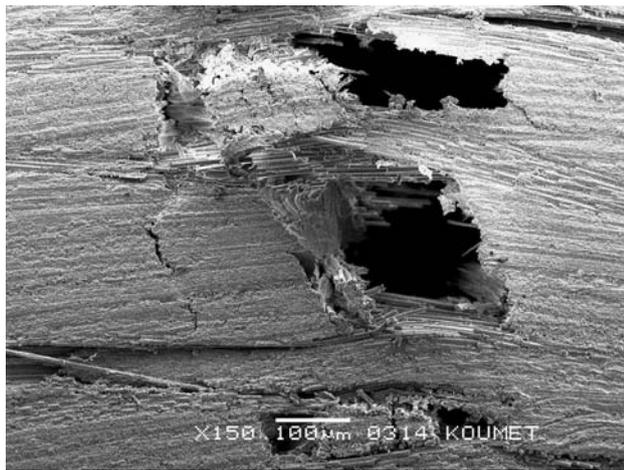
**Fig. 3** Fracture morphology of the original SBS test sample
