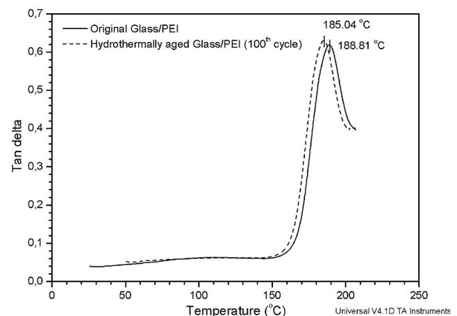
**Fig. 5** The characteristic plots of the  $\tan \delta$  versus temperature results of original and hydrothermally aged glass/PEI samples
