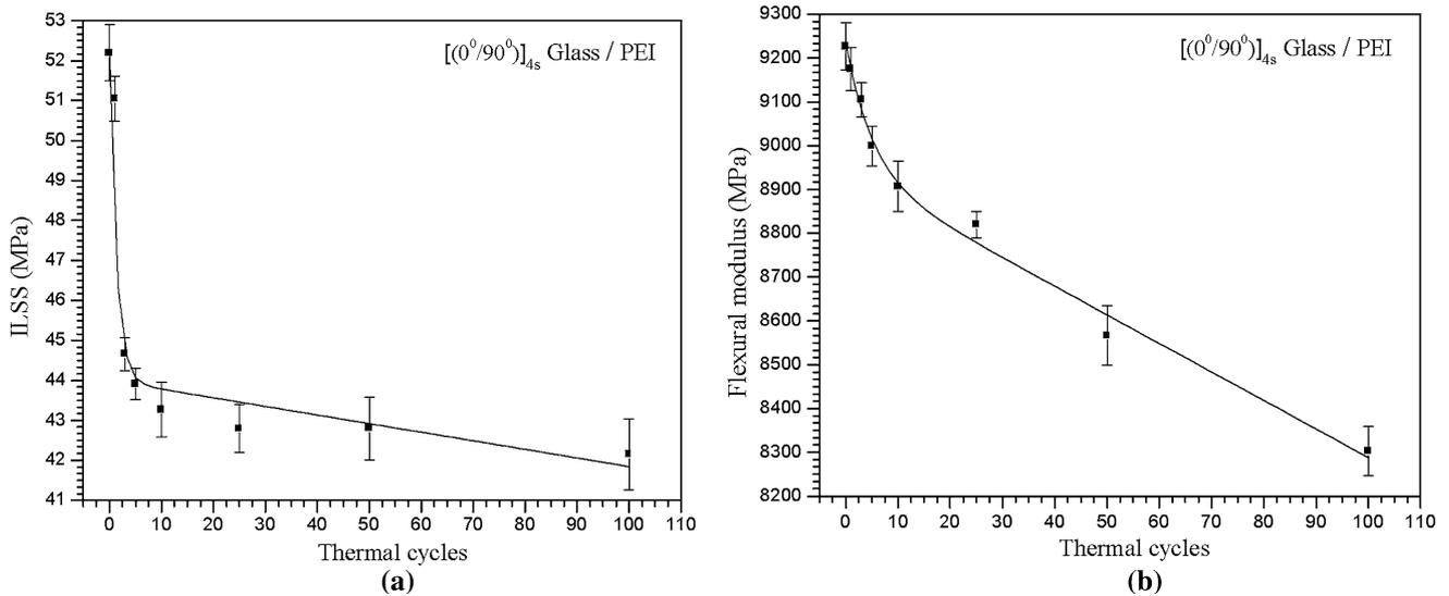
**Fig. 1** **a** ILSS versus thermal cycles results for  $[0^\circ/90^\circ]_{4s}$  glass/PEI composites. **b** Flexural modulus versus thermal cycles results for  $[0^\circ/90^\circ]_{4s}$  glass/PEI composites
