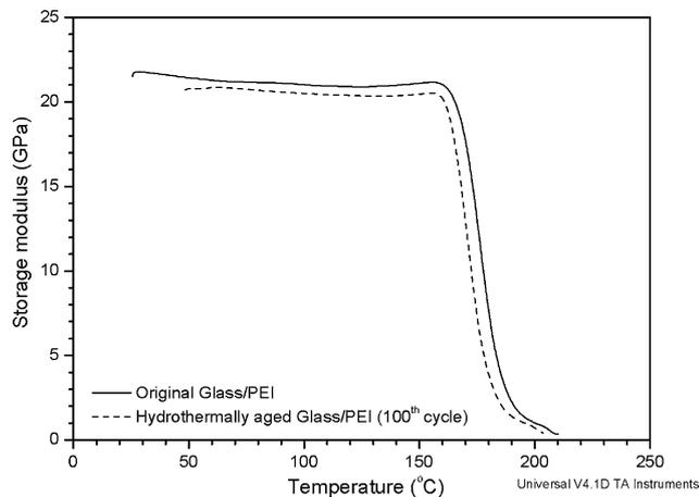
**Fig. 6** Storage modulus versus temperature results of original and hydrothermally aged glass/PEI samples
