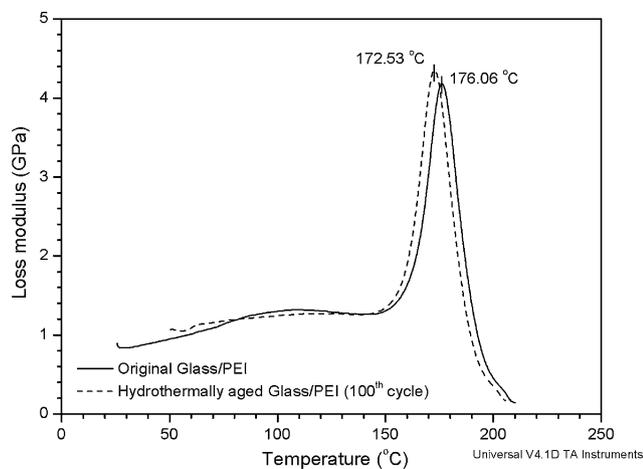
**Fig. 7** Loss modulus versus temperature results of original and hydrothermally aged glass/PEI samples
