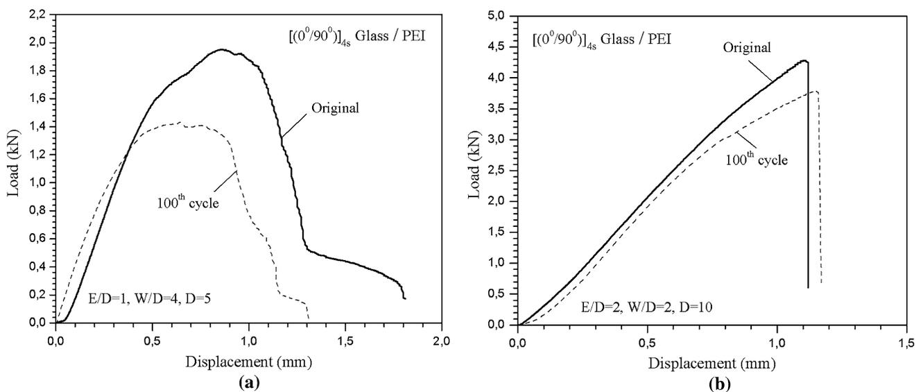
**Fig. 2** Load–displacement curves for  $[0^\circ/90^\circ]_{4s}$  glass/PEI composites with different geometric parameters
