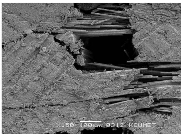
**Fig. 4** Fracture morphology of the SBS test sample exposed to 100 thermal cycles
