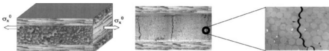
FIG. 9. Formation of cracks in transverse plies from coalescence of fiber-matrix debonds [18].
