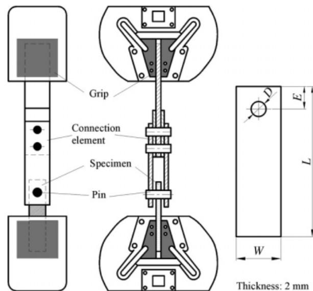
FIG. 1. Schematic illustration of the test setup for the fatigue tests of the composite pin joint.
