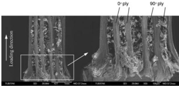
FIG. 7. The deformation types observed on the bearing plane at the edge of the pin hole.
