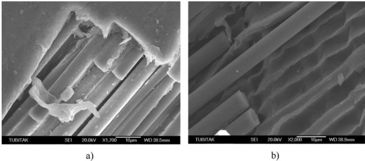
FIG. 10. Fractographic scanning electron micrographs for (a) only statically loaded and (b) firstly dynamically loaded samples.
