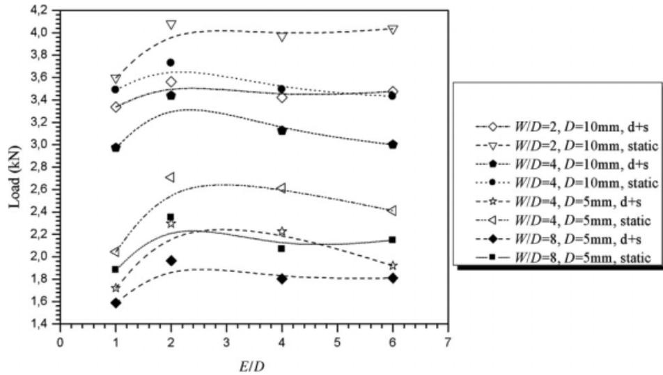
FIG. 2. Variation of the ultimate load values with respect to  $E/D$  ratio in only statically and both dynamically and SL samples.
