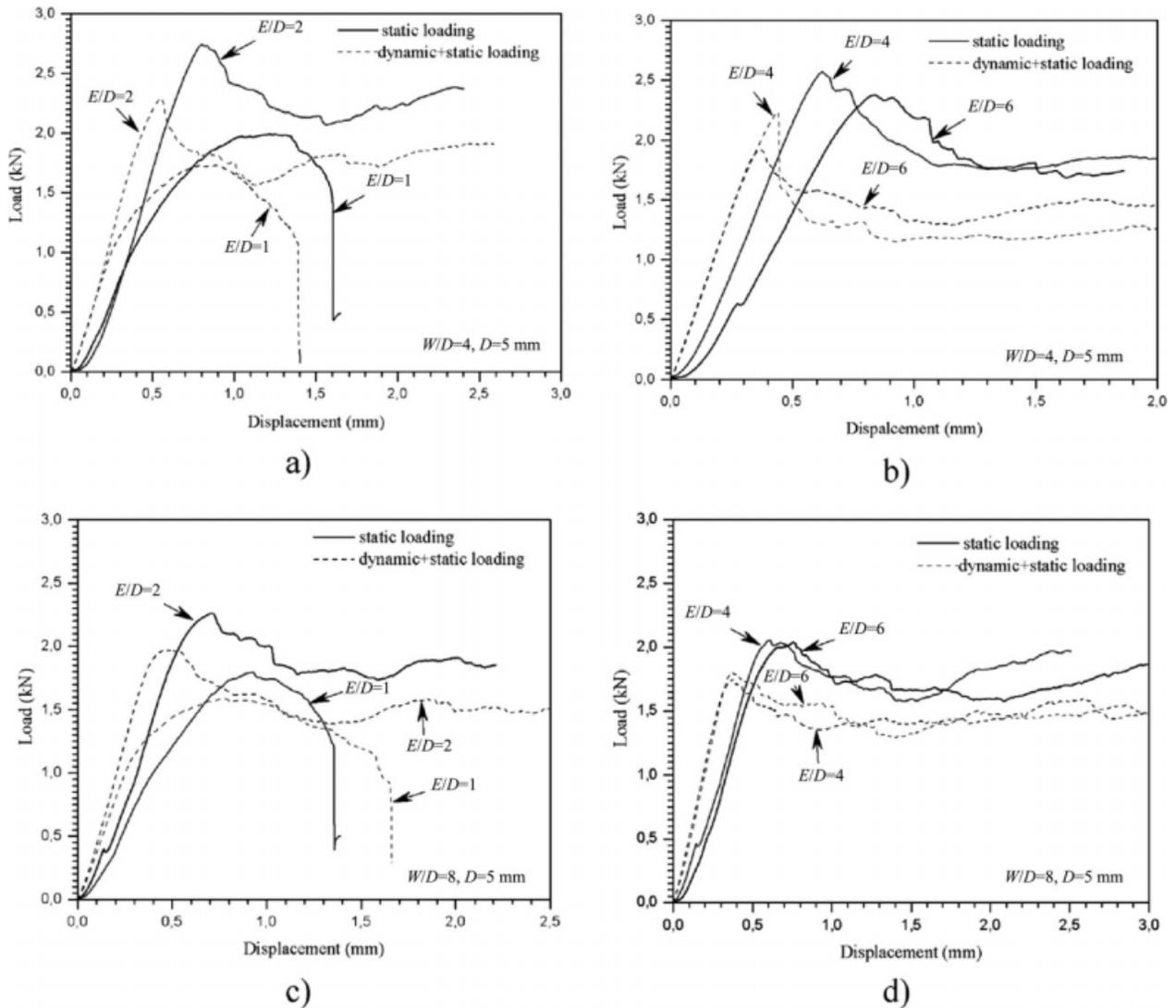
FIG. 3. Load-displacement curves for only statically loaded and firstly dynamically loaded samples ( $W/D = 4$ ,  $W/D = 8$ ,  $D = 5$  mm).
