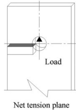
FIG. 8. The plane at which net tension failure is observed.
