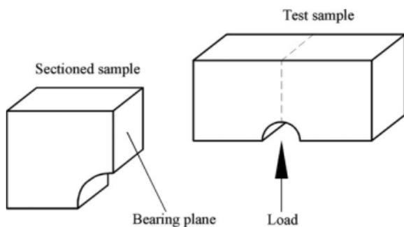
FIG. 5. Sample sectioning for determination of the bearing plane.
