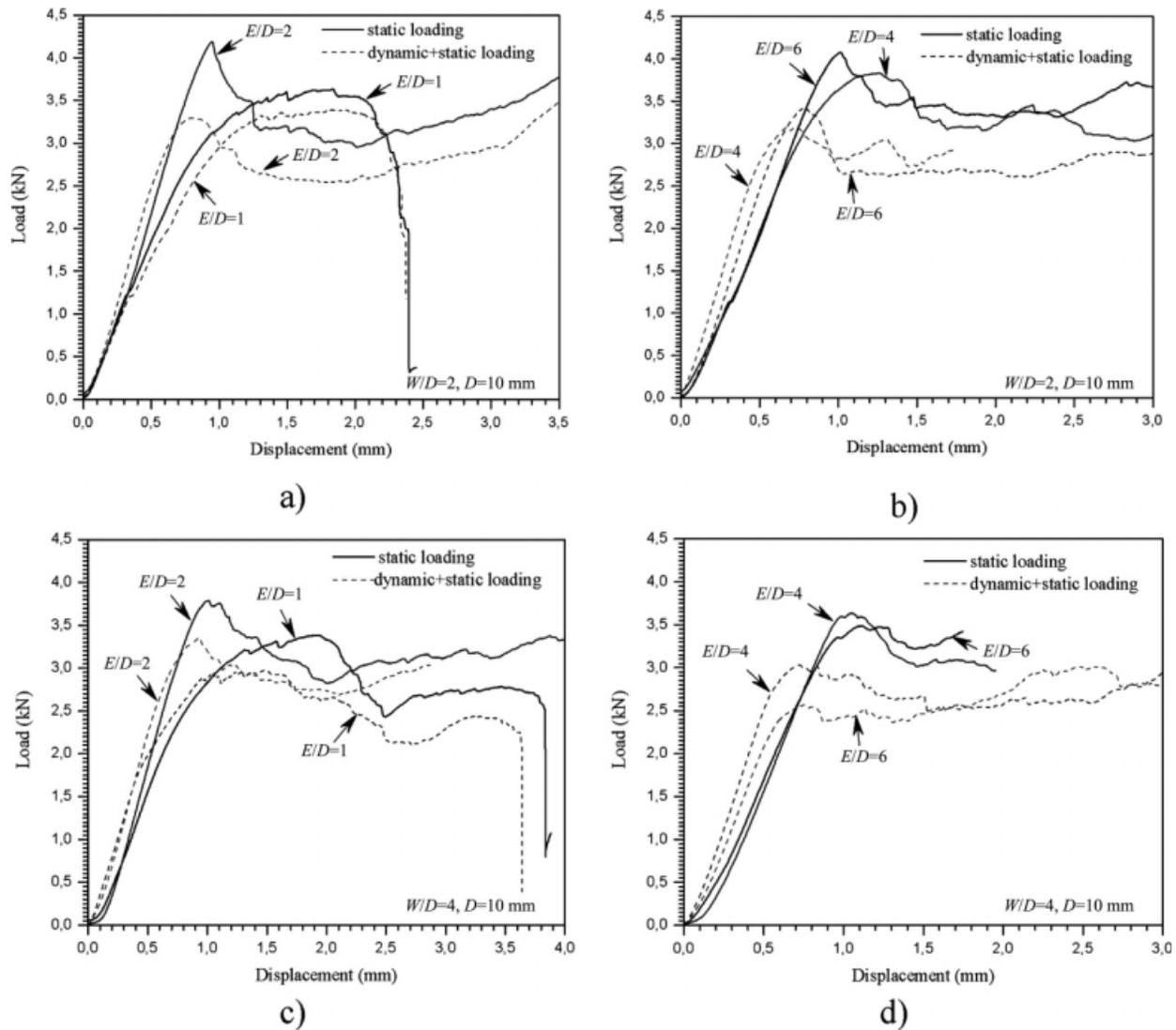
FIG. 4. Load-displacement curves for only statically loaded and firstly dynamically loaded samples ( $W/D = 2$ ,  $W/D = 4$ ,  $D = 10$  mm).
