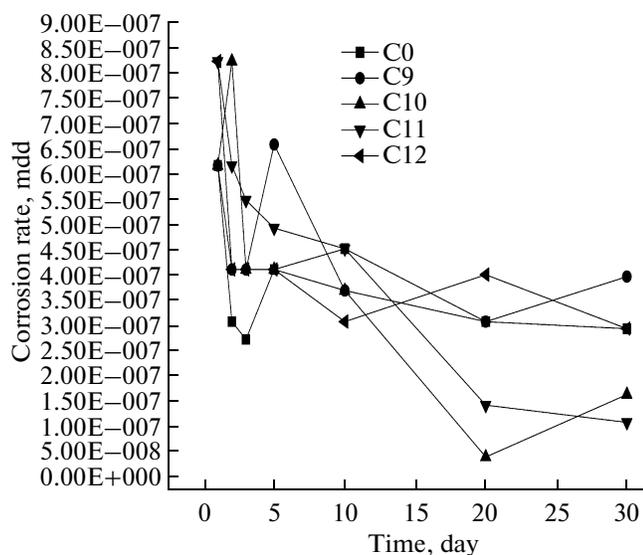
Fig. 6. Variation curve of corrosion rate of centrifugal casting G-X 10CrNiMoNb 18-10 austenitic stainless steel parts versus time.
