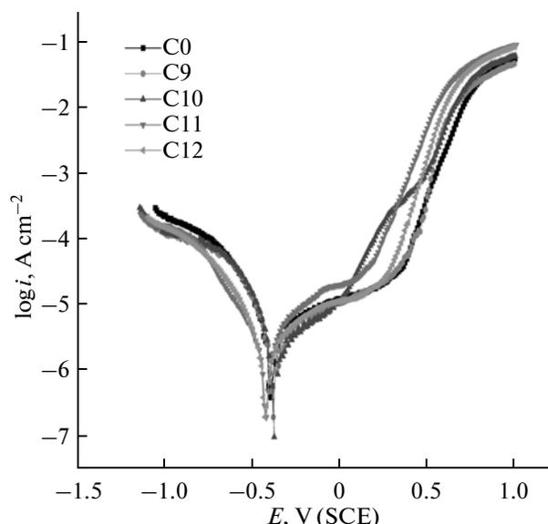
Fig. 2. Potentiodynamic polarization curves of centrifugal casting G-X 10CrNiMoNb 18-10 austenitic stainless steels.
