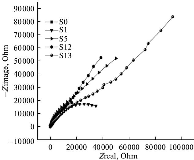
Fig. 3. Nyquist curves of sand molded G-X 10CrNiMoNb 18-10 austenitic stainless steels.
