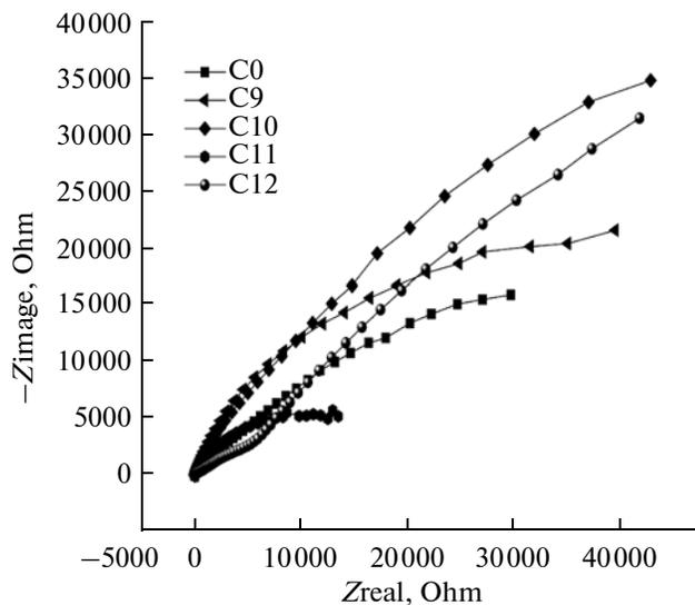
Fig. 4. Nyquist curves of centrifugal casting G-X 10CrNiMoNb 18-10 austenitic stainless steels.
