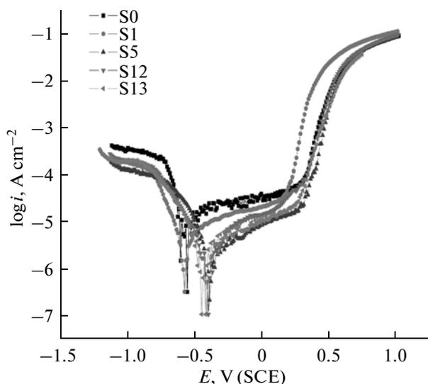
Fig. 1. Potentiodynamic polarization curves of sand molded G-X 10CrNiMoNb 18-10 austenitic stainless steels.
