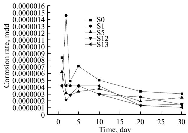
Fig. 5. Variation curve of corrosion rate of sand cast G-X 10CrNiMoNb 18-10 austenitic stainless steel parts versus time.
