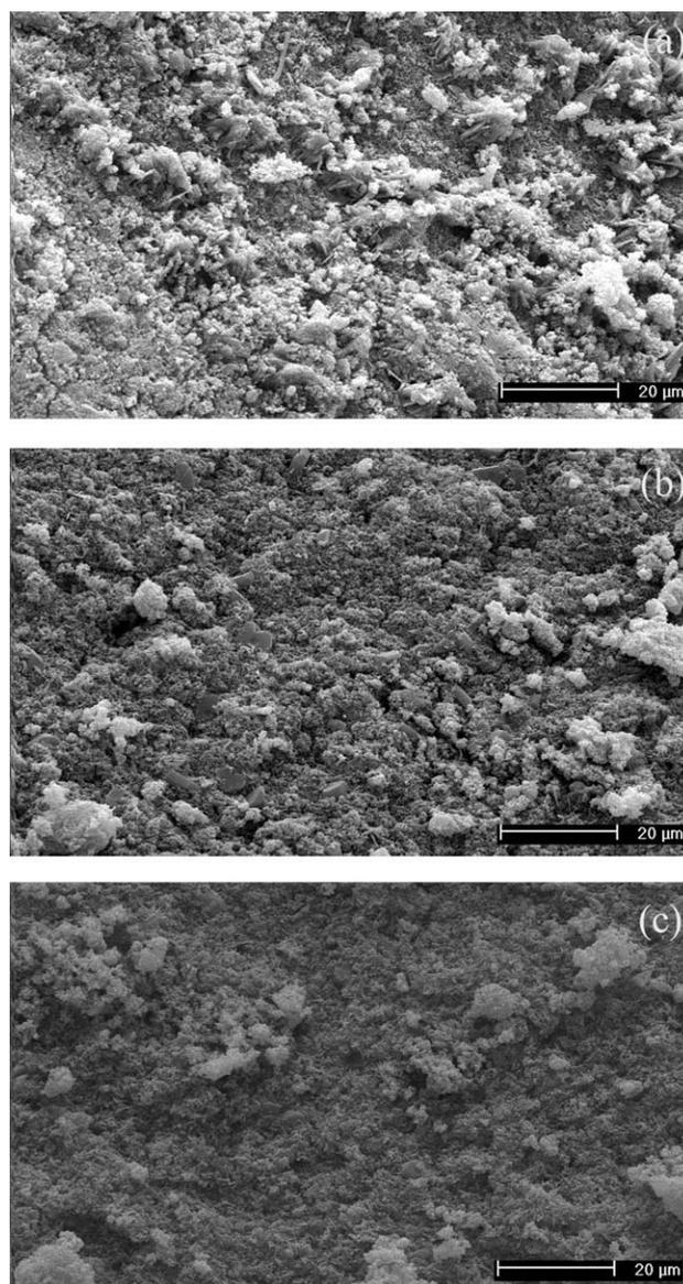
FIG. 5. Scanning electron micrographs of (a) Pure PANI, (b) PANI- $\text{CuCl}_2$  (2%), and (c) PANI- $\text{ZnCl}_2$  (2%).
