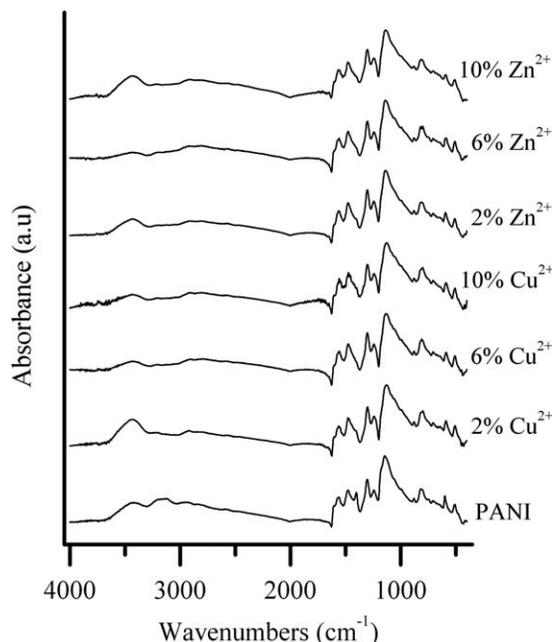
FIG. 1. FTIR absorbance spectra of  $\text{CuCl}_2$  and  $\text{ZnCl}_2$  doped PANI.
