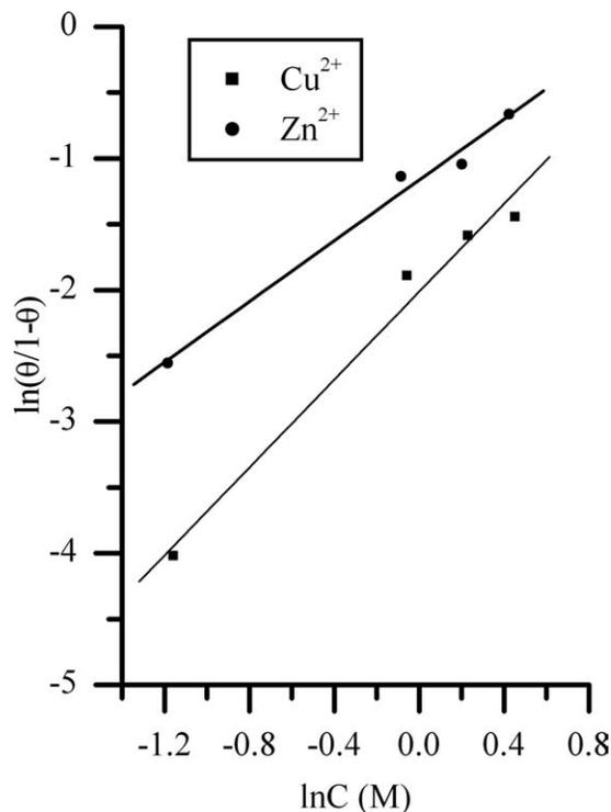
FIG. 4. Langmuir adsorption isotherm plots of PANI doped various levels of metal cations.
