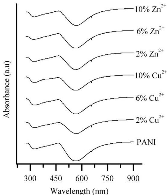
FIG. 2. UV-vis spectra of CuCl<sub>2</sub> and ZnCl<sub>2</sub> doped PANI.
