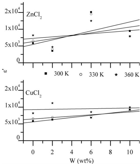
FIG. 8. Variation of real part depending on the doping level at different temperatures for 1 MHz constant frequency.
