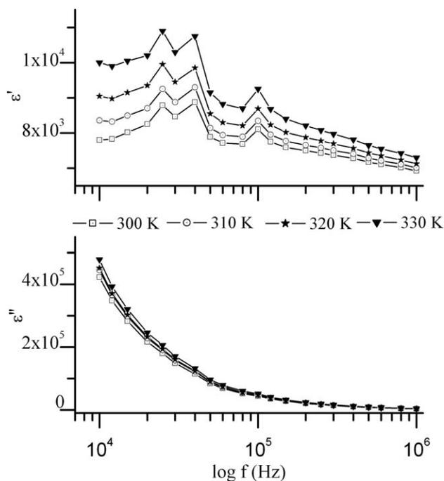
FIG. 7. Frequency dependent variations of real and imaginary parts of complex dielectric constant at different temperatures for pure PANI.
