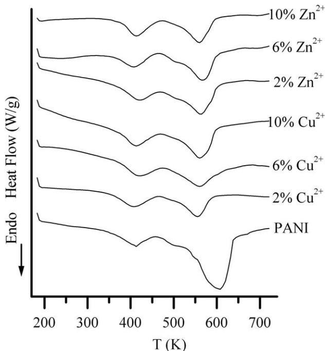
FIG. 6. DSC thermograms of  $\text{CuCl}_2$  and  $\text{ZnCl}_2$  doped PANI.
