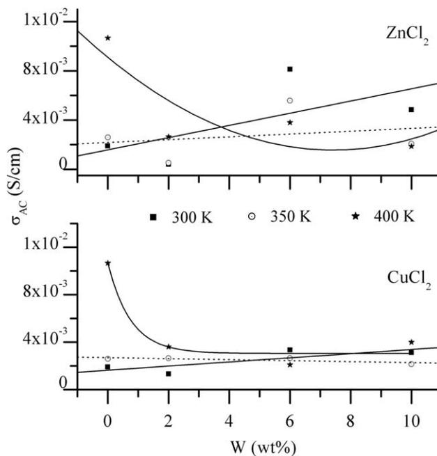
FIG. 10. Variation of ac conductivity depending on the doping level at different temperatures.
