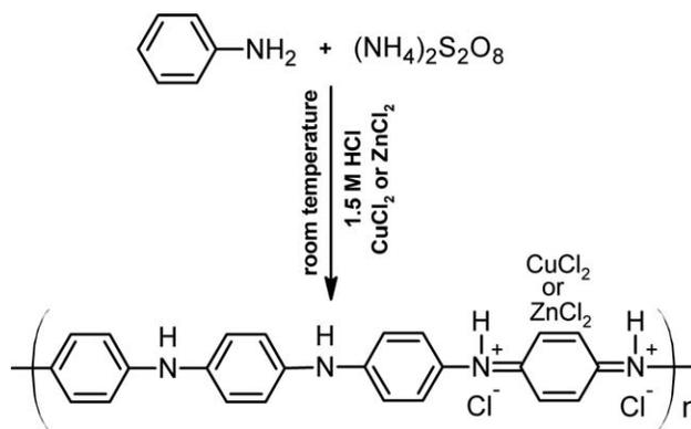
FIG. 3. The reaction mechanism of CuCl<sub>2</sub> and ZnCl<sub>2</sub> doped PANI.
